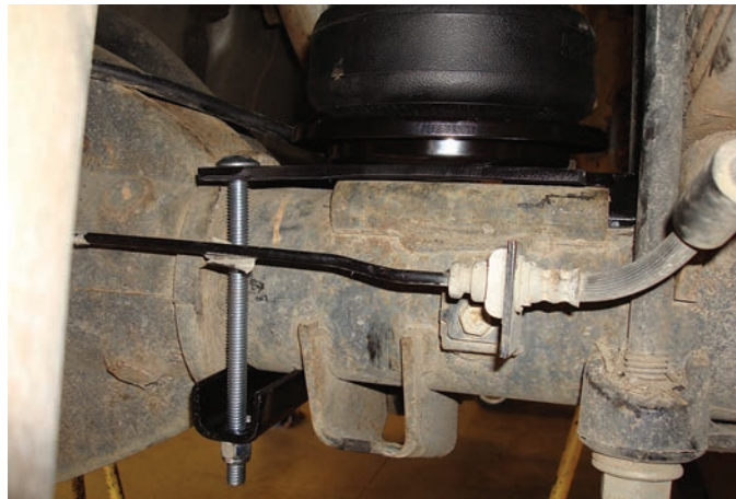
Right (passenger) side lower bracket installation
