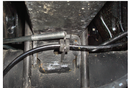
Make sure U-bolt goes between the ABS line/bracket and the leaf spring. fig. D.10
