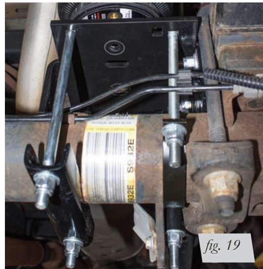
Right side (passenger) rearward axle view of finished installation torqued to 10 lb.-ft.
