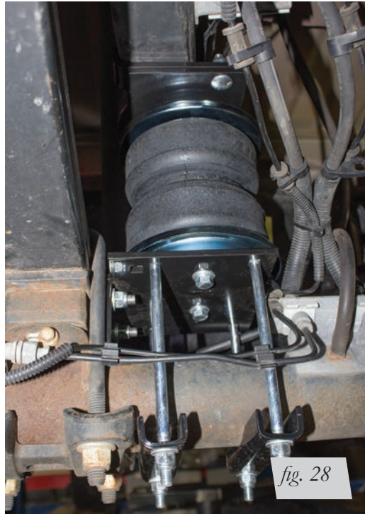
Left side (driver): rear view of installation.
