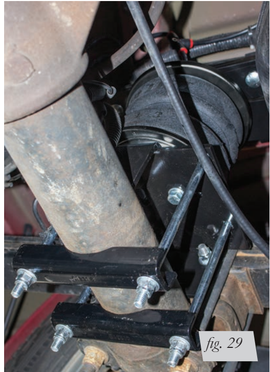
Left side (driver): front view of installation.
