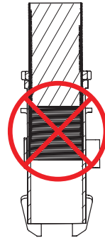
Not OK, threads are showing.
