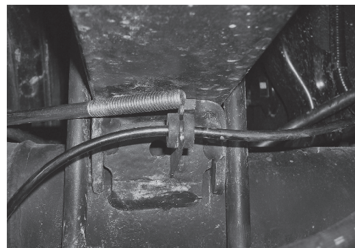
Make sure U-bolt goes between the ABS line/bracket and the leaf spring. fig. D.10
