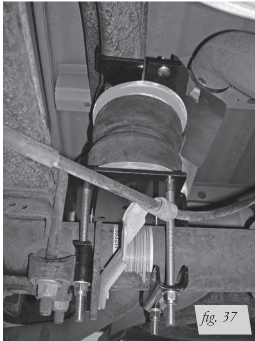
Right side (passenger): front view of installation.
