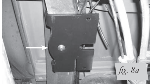
LH (driver) side. Push bracket against frame and torque to 38 lb.-ft.
