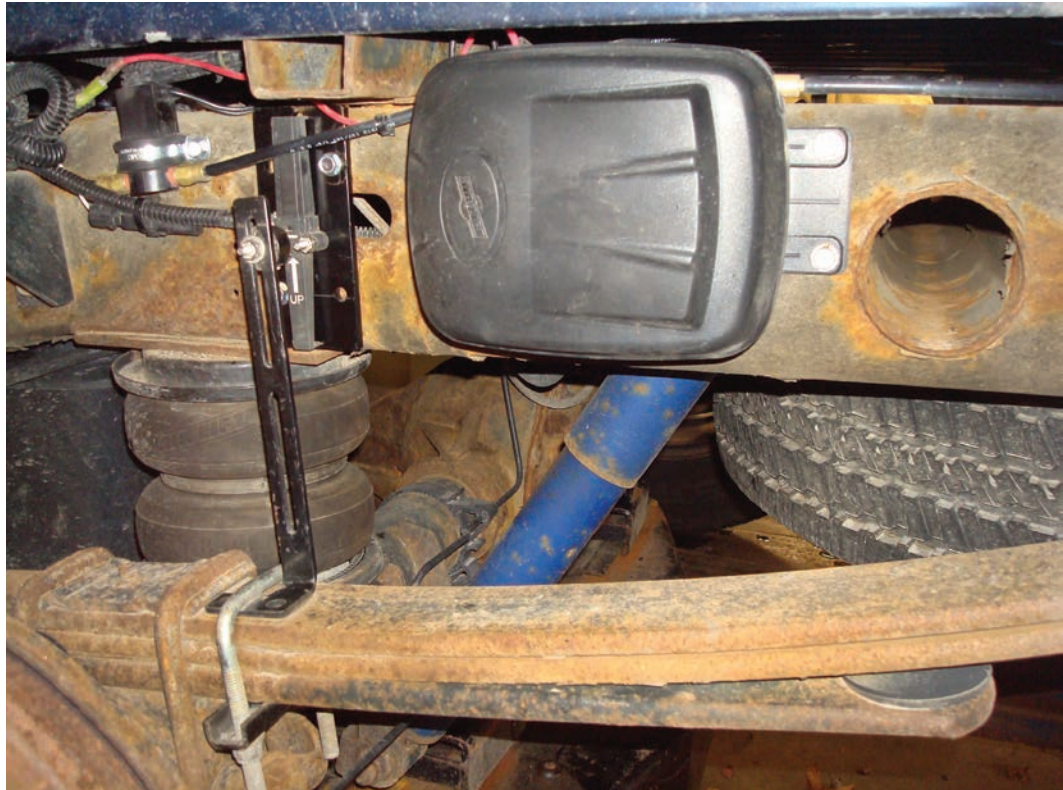
A completed install of the SmartAir II system.
