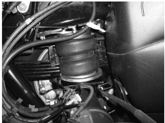
Inside, over axle view of passenger's (right) side installation.
