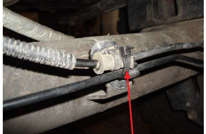
Use a zip tie and attach ABS line to brake line as shown. Fig. 11
