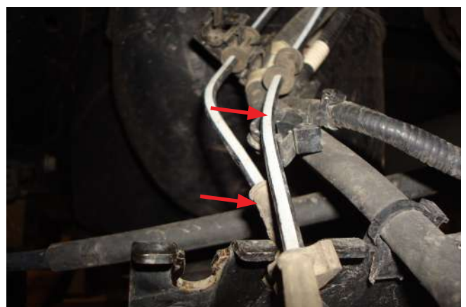
Pull the ABS lines out and away from the left side of the bracket bolted to the axle. Fig. 13
