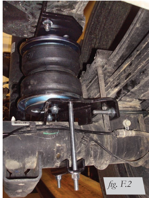
Back view of the passenger's side (right) installation.
