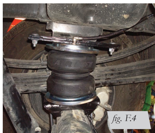
Inside view of the passenger's side installation.
