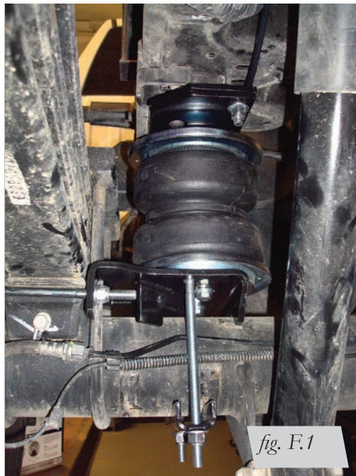
Back view of the driver's side (left) installation.
