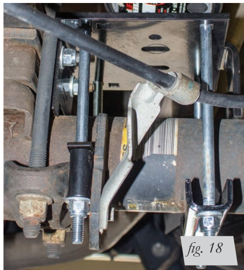
Passenger's (right) side forward axle view of finished installation torqued to 10 lb.-ft. (14Nm).
