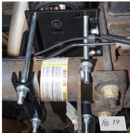
Passenger's (right) side rearward axle view of finished installation torqued to 10 lb.-ft. (14Nm).
