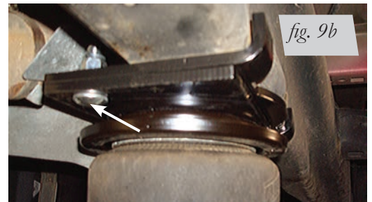
Passenger's side attached with carriage bolts (R), flat washers (M) and nylon lock nuts (U).
