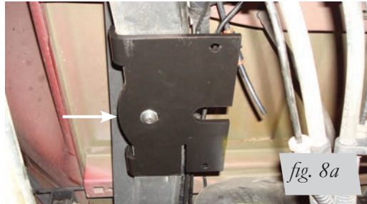
Driver's side: Push bracket against frame and torque to 38 lb.-ft. (52Nm).
