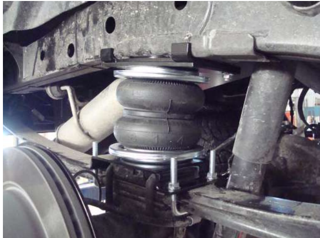
Forward, outside view of passenger's (right) side installation. Fig. 27
