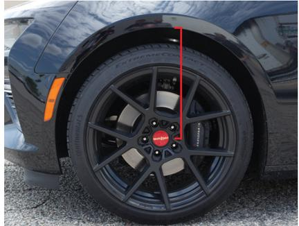
3. Add ME and MC, then divide the total by 2. Set the suspension to this point. This position will give 50% stroke in either direction and is a starting point for ride height.
