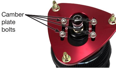
The camber plates have multiple sets of holes to allow for maximum adjustability. Use the outer holes to achieve maximum negative camber. The camber plates must always be secured with four bolts.
