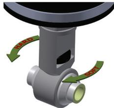
4. To adjust the dampers, start at full stiff, which is 0. Count up to keep track of, or set, the damping.
