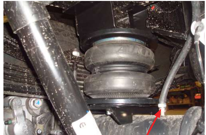
Vent tube fitting and hose
