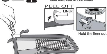
A full surface contact between tape and substrate is important for good adhesion performance. Contact is achieved by applying pressure. In practice a pressure between 40 and 50 N/cm² is usually needed and an application temperature at or above 16 °C or 60 °F is also necessary. During application, add-on parts and tapes must have the similar temperature.
