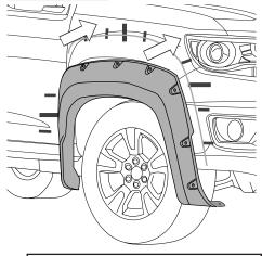
ALIGN WHEEL FLARE TOP EDGE WITH THE GREASE PENCIL HASH MARKS AND PLACE.
