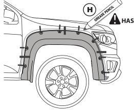
DRAW CENTER HASH MARK WITH GREASE PENCIL AT CENTER, BOTH SIDES, ON EACH SUPER-BOLT AND SHEET METAL.
