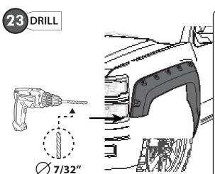
Always use extreme caution when drilling on any vehicle. Make sure that all fuel lines, brake lines, electrical wires, and other objects are not punctured or damaged when/if drilling on the vehicle.
