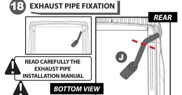
For the Right side. The exhaust pipe must be trimmed. You can place an exhaust pipe elbow coupler with a tip that poke out on the side below, or on the rear.
