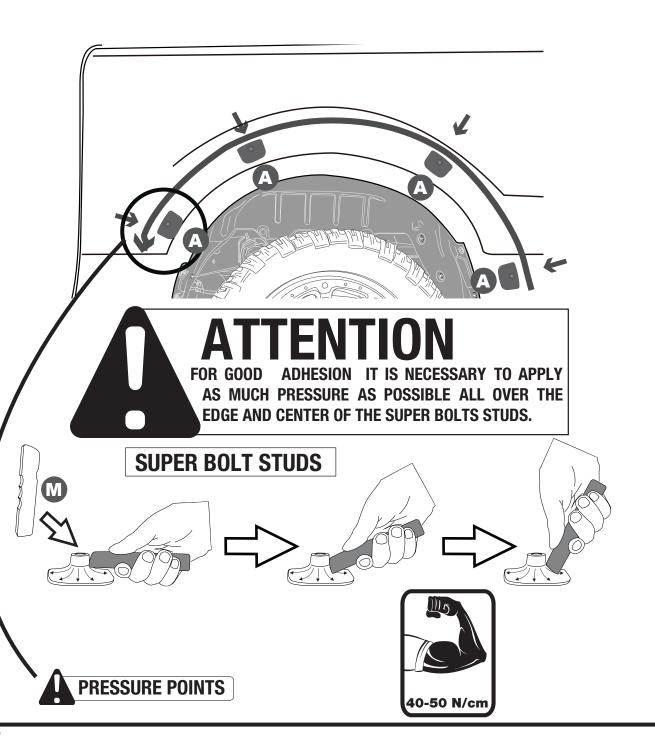
A full surface contact between tape and substrate is decisive for good adhesion performance.
