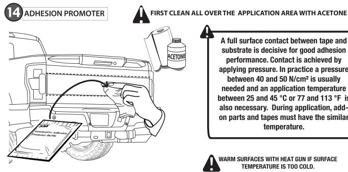
A full surface contact between tape and substrate is decisive for good adhesion performance. Contact is achieved by applying pressure. In practice a pressure between 40 and 50 N/cm<sup>2</sup> is usually needed and an application temperature between 25 and 45 °C or 77 and 113 °F is also necessary. During application, addon parts and tapes must have the similar temperature.
