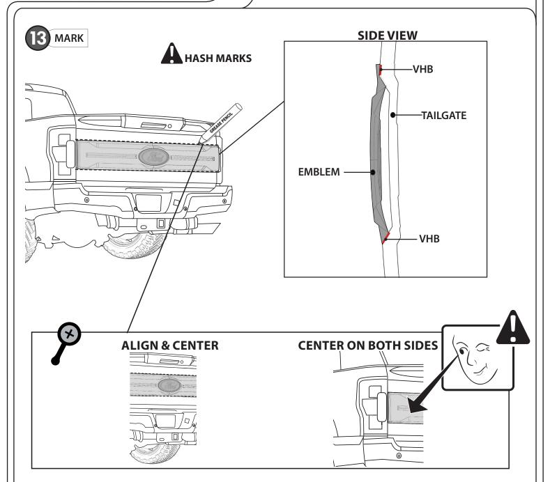
DRAW CENTER HASH MARK WITH GREASE PENCIL ON APPLIQUE AND SHEET METAL, THIS WILL ENSURE APPLIQUE WILL BE CENTERED TO **GREASE PENCIL OUTLINE.**
