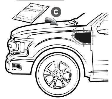
A full surface contact between tape and substrate is decisive for good adhesion performance.
