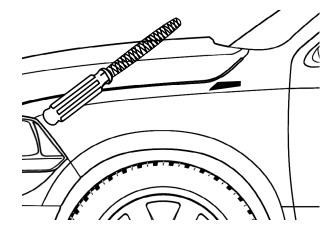
MAKE SURE FENDER VENT DON'T BIND WHEN CHECK FITTER, IF NECESSARY USE A FILE TO SMOOTH CORNERS AND EDGES UNTIL YOU HAVE CLEARANCE ALL AROUND.
