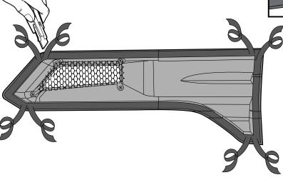
A full surface contact between tape and substrate is important for good adhesion performance. Contact is achieved by applying pressure. In practice a pressure between 40 and 50 N/cm<sup>2</sup> is usually needed and an application temperature at or above 16 °C or 60 °F is also necessary. During application, add-on parts and tapes must have the similar temperature.
