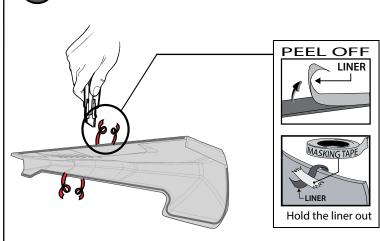
A full surface contact between tape and substrate is decisive for good adhesion performance. Contact is achieved by applying pressure. In practice a pressure between 40 and 50 N/cm² is usually needed and an application temperature between 25 and 45 °C or 77 and 113 °F is also necessary. During application, addon parts and tapes must have the similar temperature.
