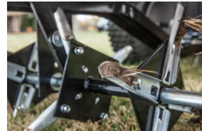
24 galvanized knives penetrate the soil easily.
