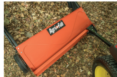
Patented off-set hitch for sweeping while you mow.
