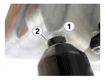
**Step 13:** Continue boring the hole (1) until the shoulder of the tool makes contact with the oil pan.
