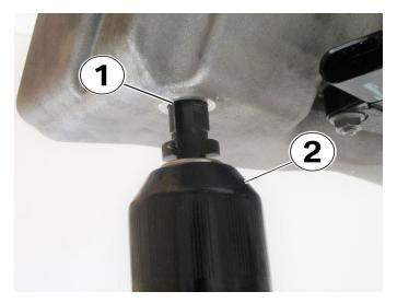
**Step 10:** Start the boring procedure. Rotate the drill (2) slowly and apply a little pressure upward into the oil pan drain plug hole.
