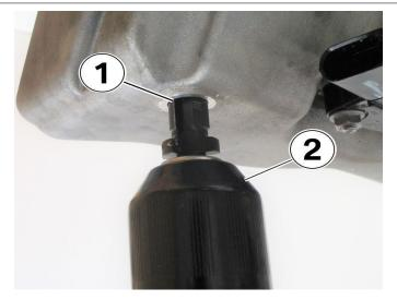
**Step 12:** When you resume boring the engine oil pan, metal chips will exit with the air pressure.
