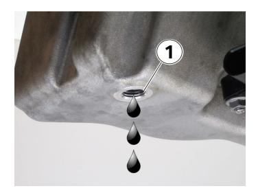
**Step 1:** Drain the engine oil (1).
