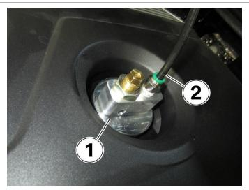
**Step 3:** Remove the engine oil cap and install the oil cap with regulator (1).
