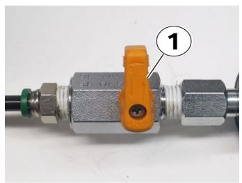
Step 2: Turn the air supply valve off (1).
