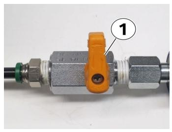
Step 7: Turn air supply valve off (1).
