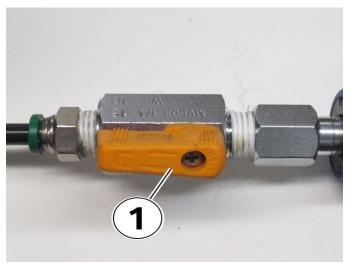
**Step 5:** Turn the air supply valve on (1).
