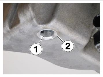
**Step 15:** Inspect the bore (1) and the chamfer (2).
