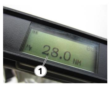
**Step 25:** Set the torque wrench to 28 Nm (20 ft-lbs).
