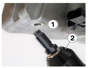
**Step 8:** Install the boring tool (1) into a suitable cordless drill (2).
