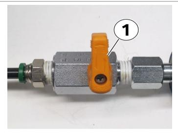
**Step 18:** After the tap is removed, turn the air supply valve off (1). Disconnect the shop air supply from the valve; the shop air supply is no longer needed.
