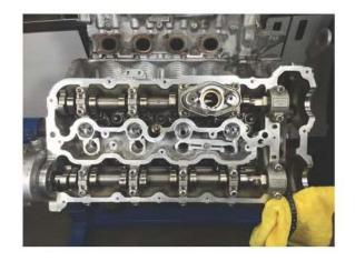
11.Loosen cam cap bolts and remove cams. Note: keep track of rocker arm location—they should not be interchanging.
