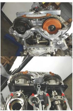
With timing chain preloaded correctly, tighten E14 M10x1 cam adjuster bolts to 30nm plus 90° clockwise on intake and exhaust.
