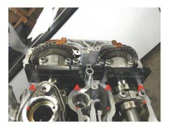
Install AGA-11-9-893-IN-N63 and install AGA-11-9-893-EX-N63 if both plates are perfectly align with cylinder head surface, then the cam timing is correct
