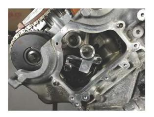
13. Transfer bolts from stock chain tensioner to chain tensioning tool (AGA-11-9-900). Tighten T40 bolts to 13nm.
