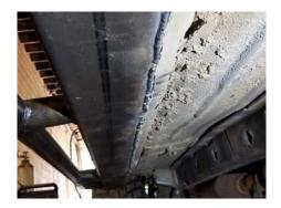
5. FULLY FINISH WELD. WELD IN 6" SECTIONS MOVING AROUND.
