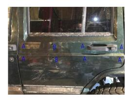
5. DRILL HOLES - 3/8" HOLES FOR BOLTS (A) AND 7/16" HOLES FOR RIVNUTS (B).
