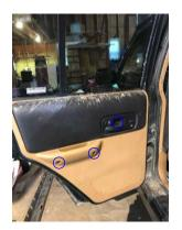
I.REMOVE (3) PHILLIPS SCREWS IN DOOR PANEL.
