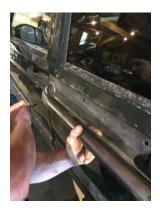
4. HOLD PANEL IN PLACE AND MARK HOLES WITH MARKER
