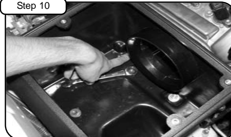
Place housing into vehicle and tighten using 12mm socket or wrench. With M8 nut and washer provided tighten down housing onto isolation mount with 13mm wrench.
