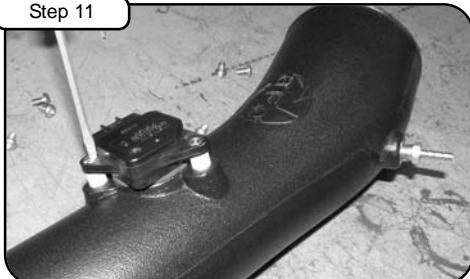
Remove MAF sensor from OE airbox using phillips screwdriver. Re-install to new aFe tube with hardware provided using flat head screwdriver (make sure gasket and nylon spacers are between tube and sensor). Install brass hose fitting.
