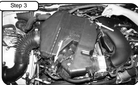
Remove engine cover with 10mm socket. With 10mm socket remove the 2 bolts holding in OE airbox. Disconnect the MAF sensor.
