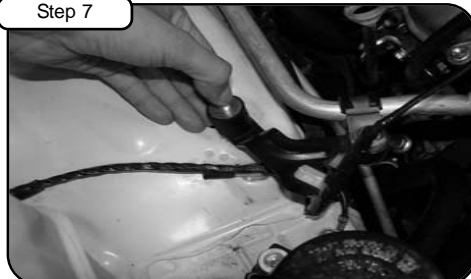
With 10mm socket and extension, remove bolt holding AC bracket. Insert M8 isolation mount and hand tighten firmly. (It may be necessary to clean the threads of undercoating or paint)
