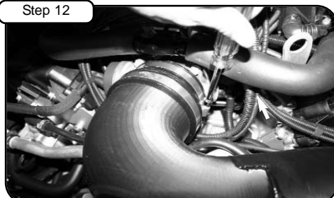
Tighten clamps using 5/16" nut driver.
