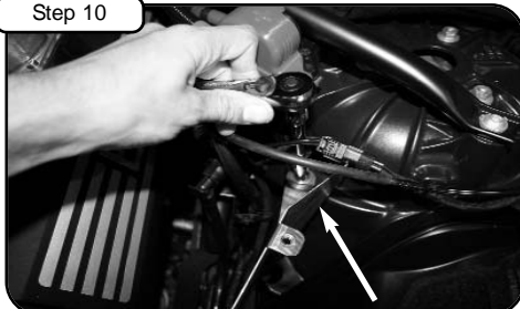
With OE T25 bolt, use to tighten new housing in to place. Tighten at bottom of housing using nut and washer provided with 10mm socket w/ extension.
