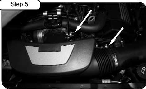
With 1/4" nut driver loosen the OE intake tube from throttle body and airbox. Remove intake tube out of vehicle.
