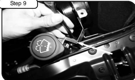
Using a 10mm wrench loosen bolt holding washer fluid reservoir. Place 5 1/2" adapter in to new housing and tighten using button head screws provided with 5/32 allen key. Install housing in to vehicle and re-tighten bolt.
