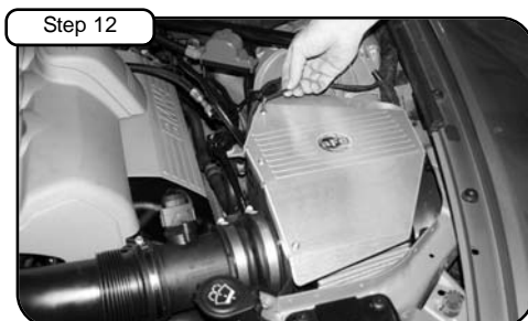
Install cover on housing using button head screws provided and tighten using 5mm allen key.
