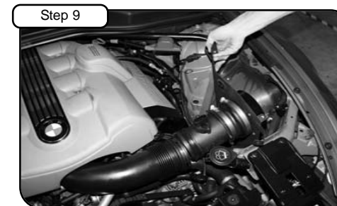
Place MAF sensor into intake tube. (Make sure MAF sensor arrow is in direction towards throttle body.) Now install housing into vehicle. Place other end of MAF sensor into coupler. Do not tighten clamps.
