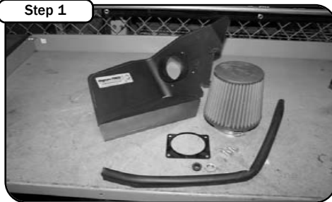
Step 1 Complete kit. Make sure all components are present prior to beginning installation.
