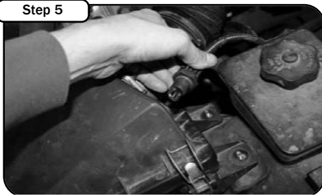
Step 5 Remove the factory air temp sensor. Set aside for re-installation.
