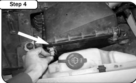
Step 4 Unclamp the 2 factory airbox clips.
