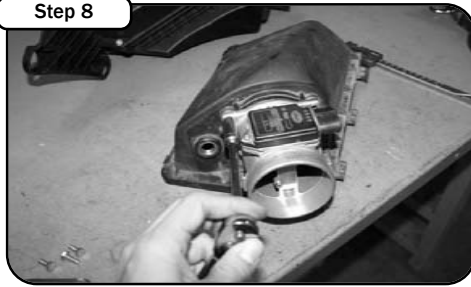
Step 8 Using a 10mm socket, unscrew the 4 factory screws securing MAF sensor. Disconnect the MAF sensor and transfer onto new housing using new gasket provided.
