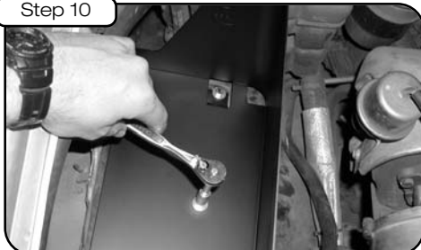
Using remaining M8 hardware and the existing holes in the fenderwell, secure the heat shield to the fender well. Tighten the hardware.
