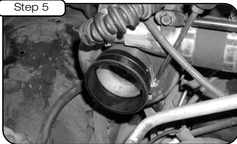
Place provided coupler onto turbo and secure the turbo end by tightening provided clamp.
