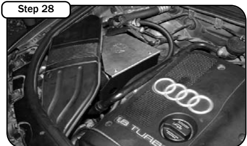
Step 28 Your installation is now complete. Make sure you check that all clamps and electrical connections are tight. Re-check periodically.
