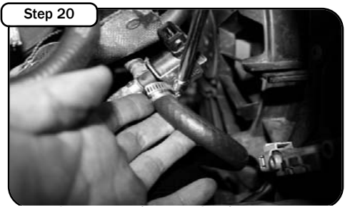
Step 20 Use provided 8.5"L x 3/8" hose with 3/8" elbow and clamp. Install onto second from bottom fitting. Tighten clamp onto factory switch valve. Verify plug is reconnected.
