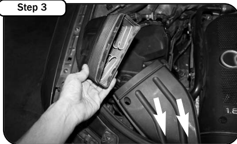
Step 3 a. Remove two screws holding factory fresh air duct in place. b. Pull fresh air duct out of vehicle and save for later use
