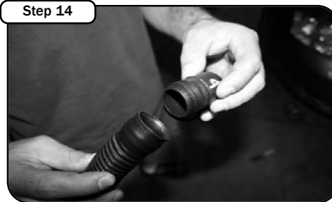
Step 14 Remove fitting from air pump hose and install provided breather filter. Install filter onto air pump and replace fog lamp and grill.
