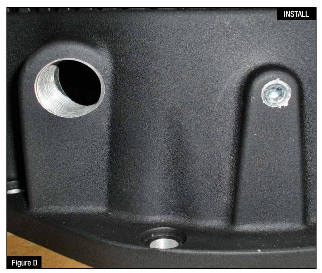
**Refer to Figure D for step 9** (Skip this step if you are going to install a temperature sensing unit) Step 9: Install 1/8" NPT plug on top of aFe differential cover (torque to 30 in. -lbs.).
