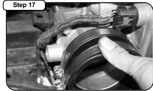
Step 17 Install supplied coupler and clamps on throttle body, do not tighten
