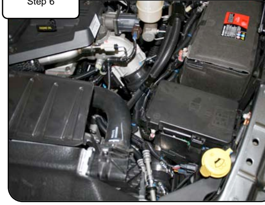
Install new tube and position into coupler on manifold. Tighten and torque all four clamps to 75 in-lbs. Check and tighten after 50 miles! Your Intercooler tube installation is now complete. Thank you for choosing aFe power!
