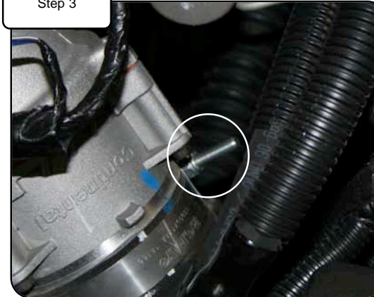
With 7/16" deep socket, loosen clamp on manifold. Push down on intercooler tube and disconnect from manifold. Remove stock intercooler tube from vehicle.
