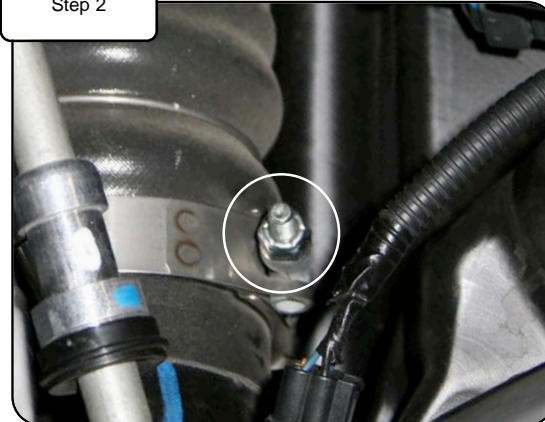
With 7/16" deep socket, loosen clamp on intercooler.
