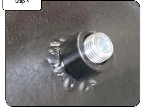
Install plugs in to 1/8" NPT ports with 3/16" hex key.
