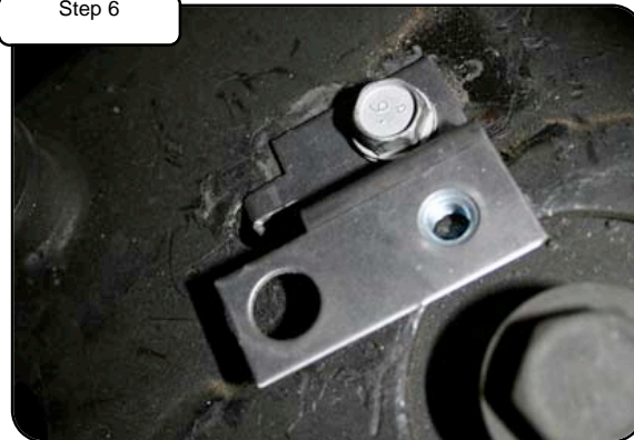
Remove brake line bracket from the frame at fender well using 13mm socket. Install bracket adapter supplied with original screw.
