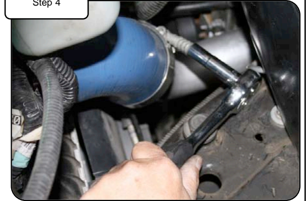
Loosen clamps on the intercooler elbow coupler using 7/16" deep socket with extension.
