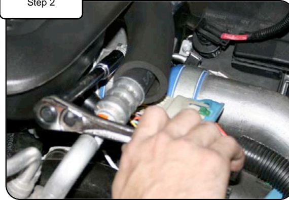
Loosen clamps on the turbo outlet using 7/16" deep socket or wrench. Do not damage the clamp to the turbo housing, as it will be re-used.
