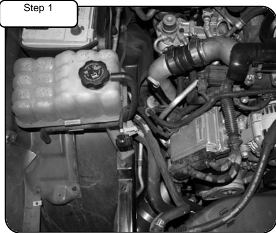
Complete Stock Intercooler tube. (Note: the air intake system has been removed)
