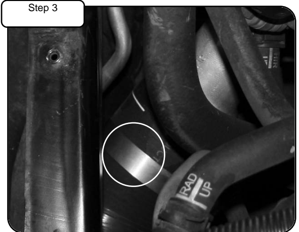
With 7/16" deep socket, loosen clamp on intercooler coupler. Push down on intercooler tube and disconnect from manifold. Remove stock intercooler tube from vehicle.
