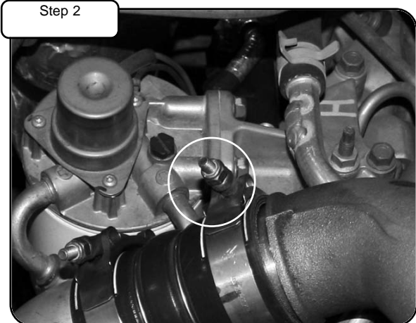
With 7/16" deep socket, loosen clamp on manifold.
