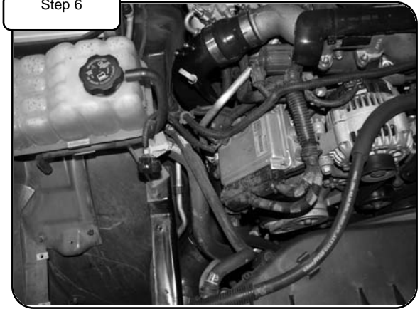
Install new tube and position into coupler on intercooler. Tighten and torque all clamps to 75 in-lbs.. Reinstall the air intake system and your intercooler tube installation is now complete. Thank you for choosing aFe power!
