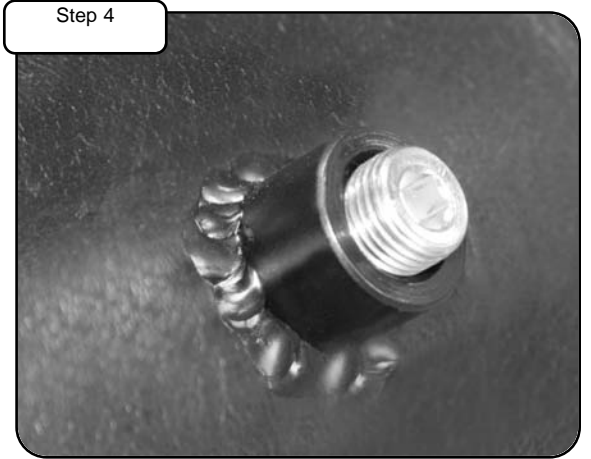
Install plugs in to 1/8" NPT ports with 3/16" hex key. Use teflon pipe sealant tape for leak tight fit.
