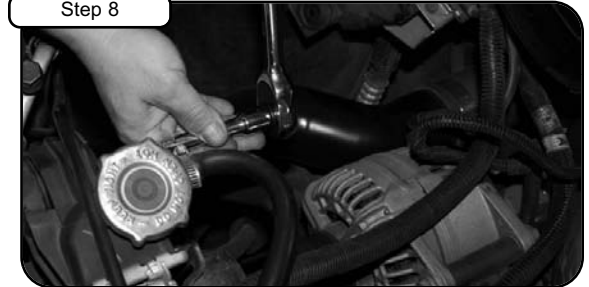
With 10mm socket and extension loosen the two bolts holding in radiator on back of upper radiator support.
