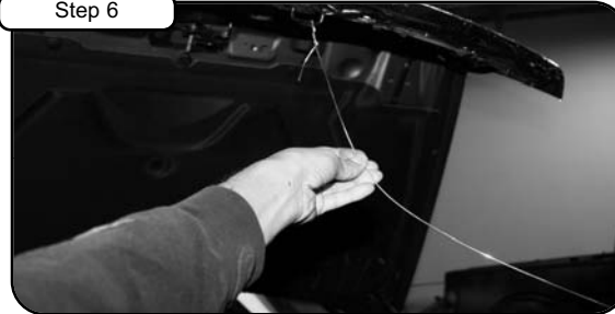
With A/C condensor turned 90 degrees, secure to the vehicles lifted hood using steel wire.
