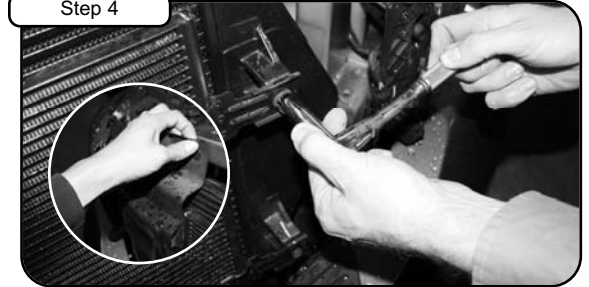
Remove plastic A/C line protector on passenger side. With 13mm socket or wrench loosen the 4 bolts holding in A/C condensor.
