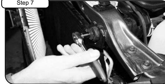
With 10mm socket or wrench remove the 2 top intercooler attachment bolts connected to upper radiator support.
