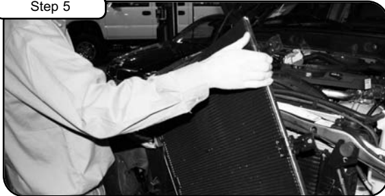
Rotate the A/C condensor up and out away from vehicle. Take care to prevent damage to A/C lines.
