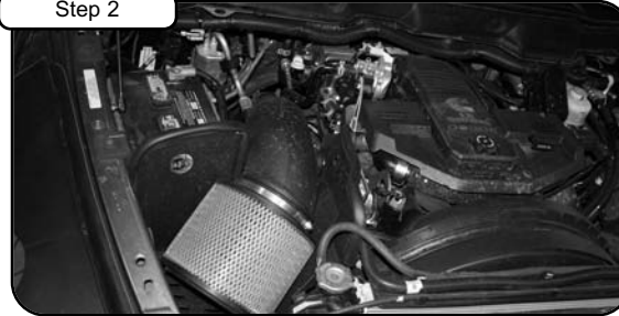
Disconnect battery before install. Remove stock air box or intake system from vehicle for easier installation.
