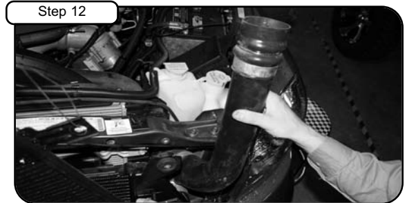
Remove stock intercooler outlet tube from vehicle.
