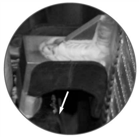
Position and make sure intercooler rubber U-shaped isolators sit square on cross beam and have not folded during installation.
