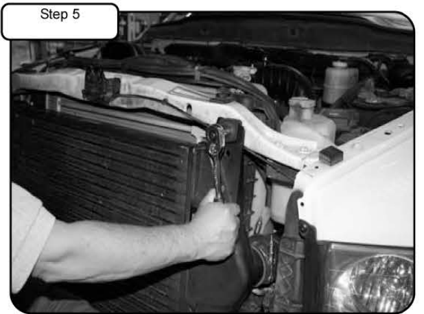
Step 5 With 10mm socket or wrench remove the 2 top intercooler attachment bolts connected to upper radiator support.
