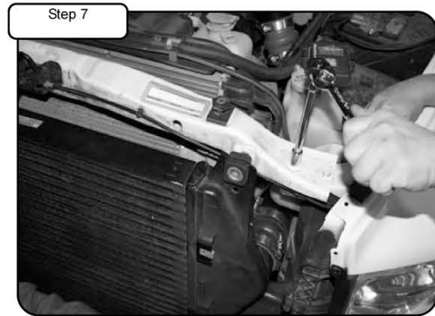
Step 7 Loosen and remove the 4 bolts holding in upper radiator support using 13mm socket or wrench.
