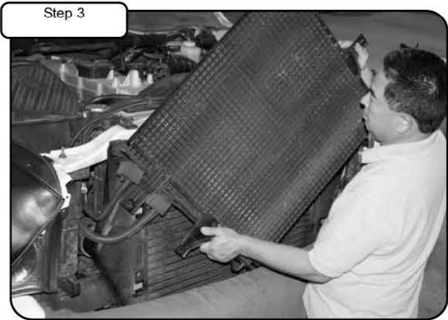
Step 3 Rotate the A/C condenser up and out away from vehicle. Take care to prevent damage to A/C lines.
