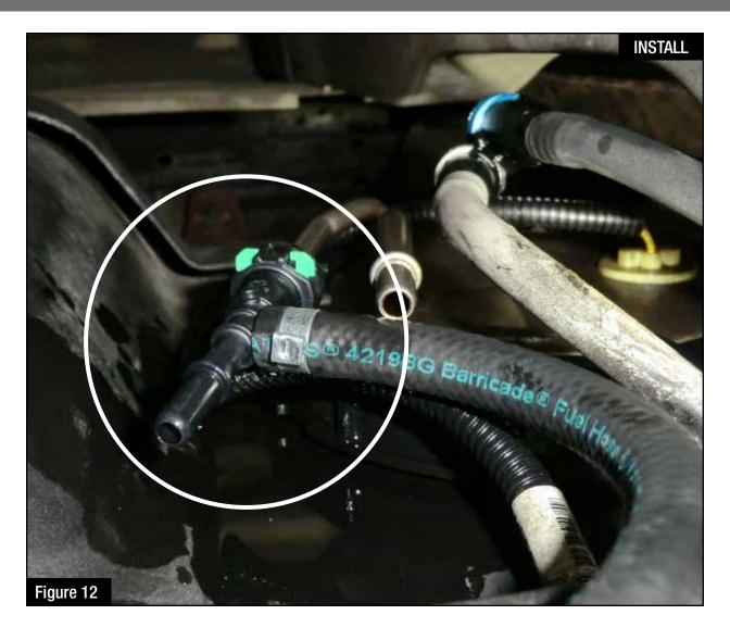
Step 12: Install the supplied fuel return line to the male side of the stock return fuel line on the tank and lock the fitting.
