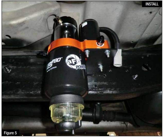
Step 7: Using a light oil, lube the gasket on the fuel filter and install on the manifold. Thread the supplied water separator bowl onto the supplied fuel filter.
