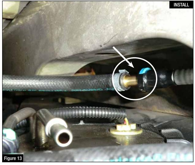
Step 13: Install the supplied fuel outlet hose (Shown below with black 90° "AN" fitting) onto the female side of the stock fuel line.
