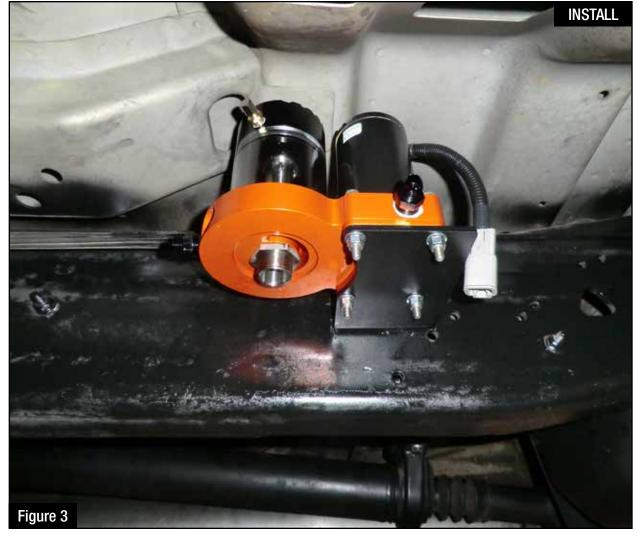
Step 4: Connect the manifold to the bracket using the four (4) supplied M6x1.0 x 50mm bolts, M6 washers, fiber washers and M6 flange nuts. The fiber washers go between the manifold and the bracket.
