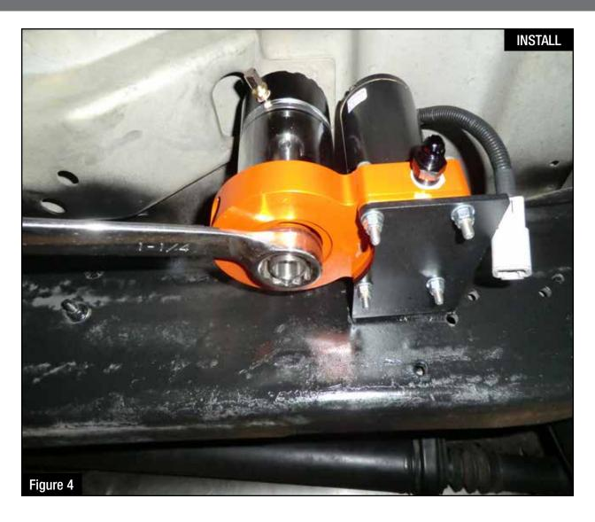
Step 6: Turn the sight glass to the desired angle and using a 1-1/4" wrench, tighten the center nut under the DFS780 manifold.
