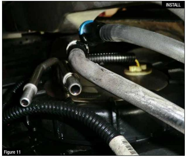
Step 11: Disconnect the fuel supply and the fuel return line.
