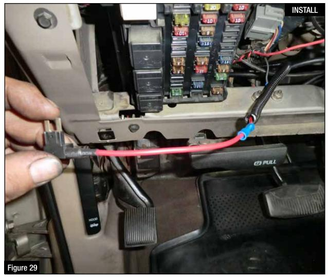
Step 33: Attach the power wire from the relay to the inline fuse adapter.
