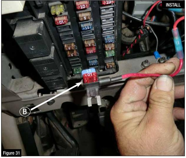
Step 35: Install the fuse removed in Step 34 and insert it into the open location on the fuse adapter B (not in line with the wire).
