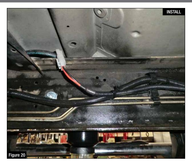
Step 20: From the inside of the frame, plug the Deutsch connector of the supplied wiring harness into the mating connector on the DFS780.
