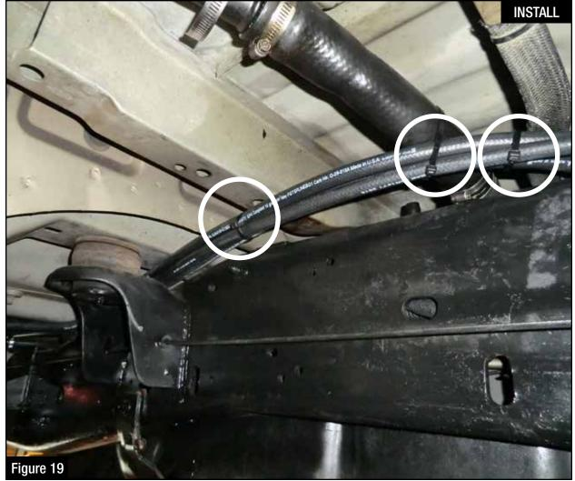
Step 19: Using the supplied nylon cable ties, secure the new hoses (as shown above).
