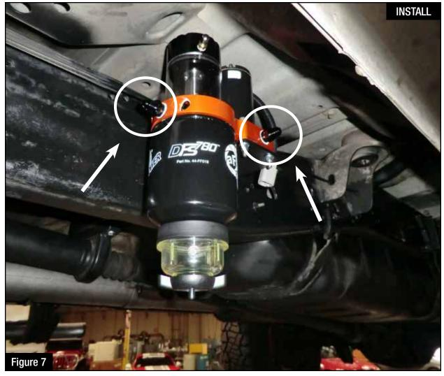
Step 9: Install the 2 x 3/8" NPT to -6 AN fittings into the DFS 780 (as shown above)
