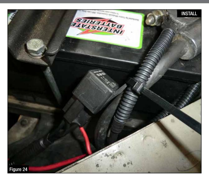
Step 26: Secure the supplied relay using a supplied nylon cable tie.
