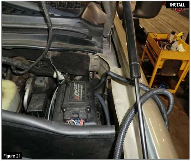
Step 23: Run the other end of the supplied wiring harness along the frame to the engine compartment. Secure using supplied nylon cable ties.
