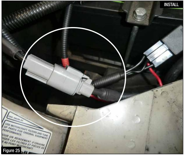
Step 27: Plug the supplied relay harness into the Deutsch connector on the power harness. Step 28: Organize any of the loose wire harness and secure with the remaining nylon cable ties.
