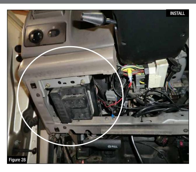
Step 32: Locate the under dash fuse box.
