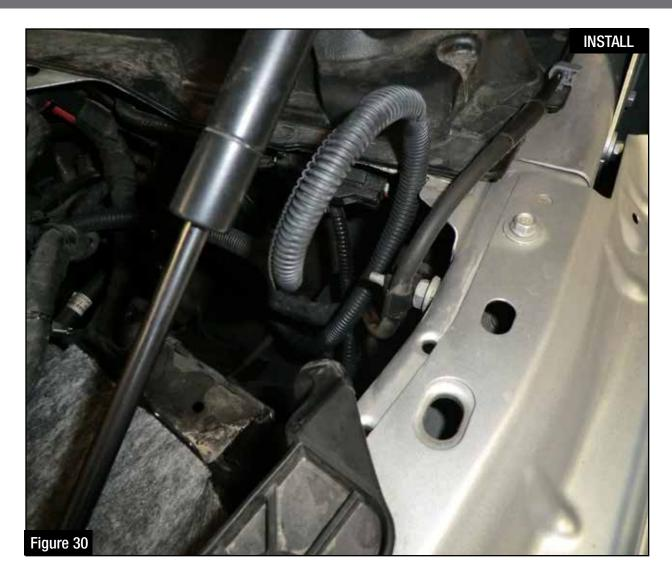
Step 45: Run the remaining wire harness along the frame to the engine compartment. Secure using supplied nylon cable ties.
