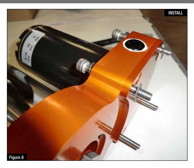
Step 9: Install the four (4) supplied M6x1.0 x 50mm bolts, M6 washers, and fiber washer. The fiber washers go between the DFS780 manifold and the bracket.
