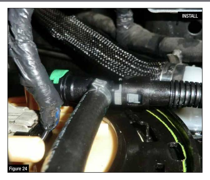
Step 35: Connect the factory fuel return line (female connection) onto the tee fitting at the end of the supplied fuel return line (male connection).
