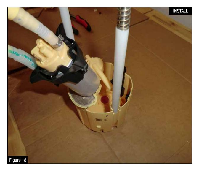
Step 24: Remove the fuel pump, fuel feed and fuel return line from the fuel pump sender assembly.
