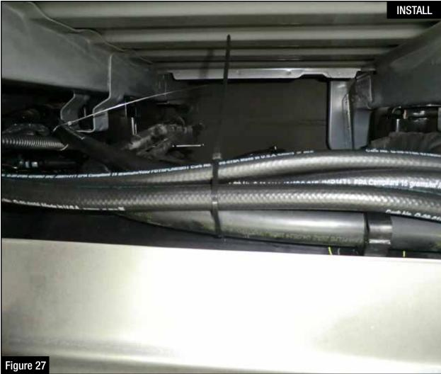
Step 39: Route the hoses as shown and secure with the supplied nylon cable ties.
