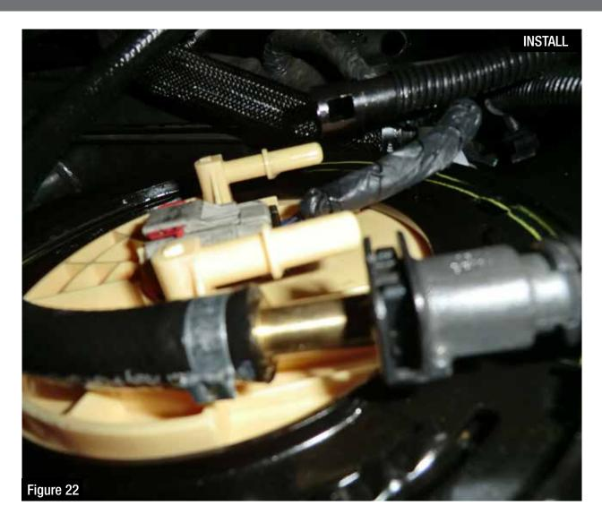
Step 32: Install the 3/8" quick disconnect fitting (male connection) on the supplied fuel outlet hose into the quick disconnect fitting (female connection) on the stock fuel feed line.
