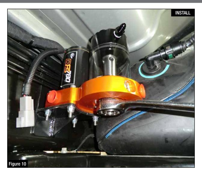
Step 11: Turn sight glass to the desired angle. Using a 1-1/4" wrench, tighten the center nut under the DFS780 manifold.
