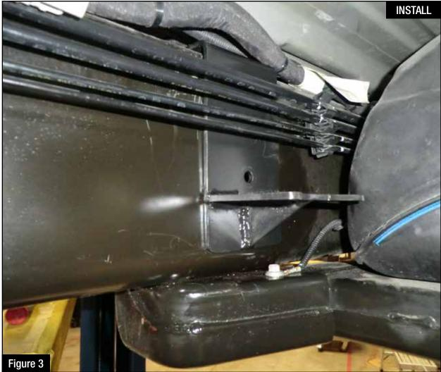
Step 3: Place the supplied bracket between the frame and the hard lines. Step 4: Line up the bracket with the hole located in Step 1.
