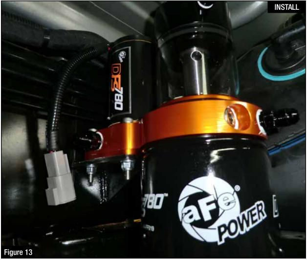
Step 14: Install the 2 x 3/8" NPT to -6 AN fittings into the DFS780 manifold (DO NOT overtighten).
