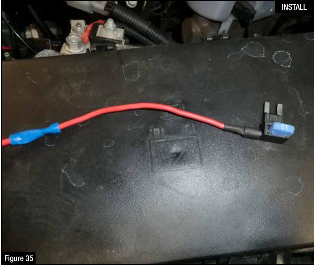
Step 51: Attach the power wire from the relay to the inline fuse adapter.
