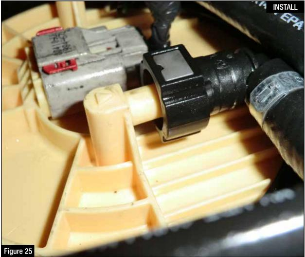
Step 36: Install the 90° 3/8" quick disconnect fitting (female connection) on the supplied fuel inlet hose onto the quick disconnect fitting (male connection) on the fuel pump sender assembly.Step 37: The fuel line should point towards the center of the vehicle.
