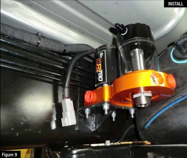
Step 10: Connect the DFS780 manifold to the bracket using the four (4) supplied M6 flange nuts (make sure the fiber washers isolate the pump body from the bracket).
