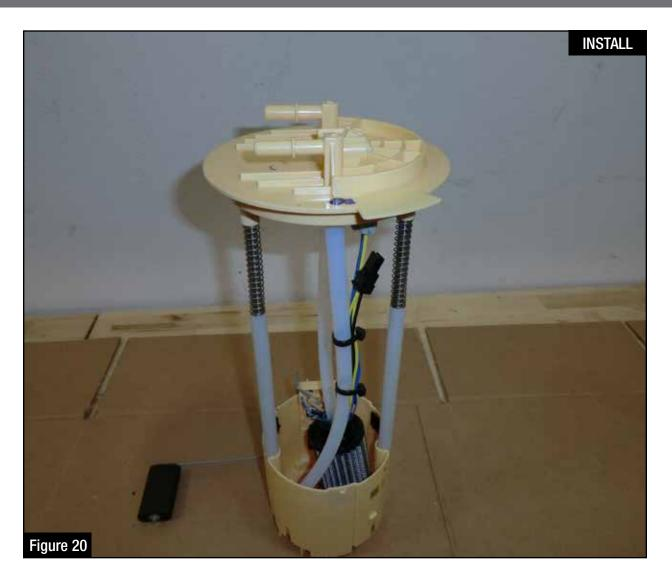
Step 27: If the fuel level sending unit was removed, reinstall at this time.
