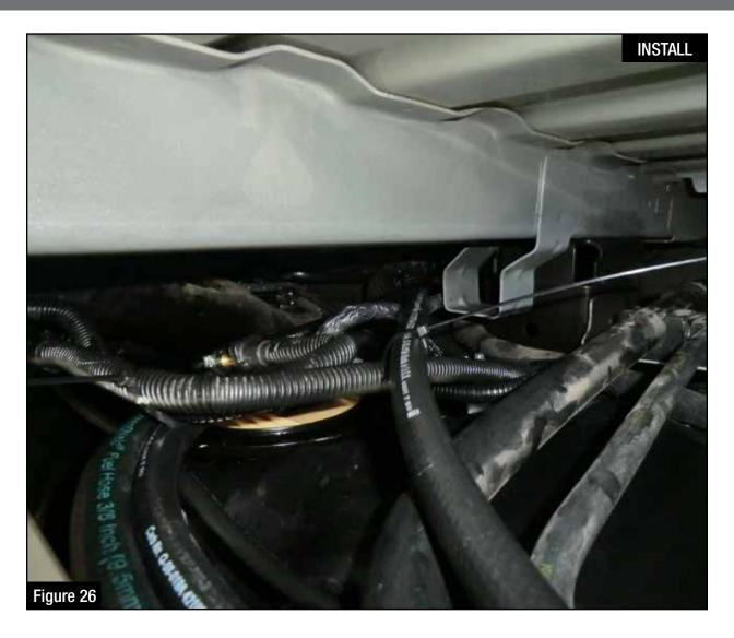
Step 38: Route the hoses as shown and secure with the supplied nylon cable ties.
