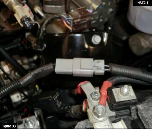
Step 48: Plug the supplied relay harness into the Deutsch connector on the power harness. Step 49: Organize any of the loose wire harness and secure with supplied nylon cable ties.
