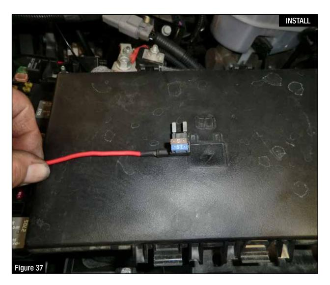
Step 53: Using the supplied inline fuse adapter, install the fuse removed in Step 52 and insert it into the open location on the fuse adapter (not in line with the wire).
