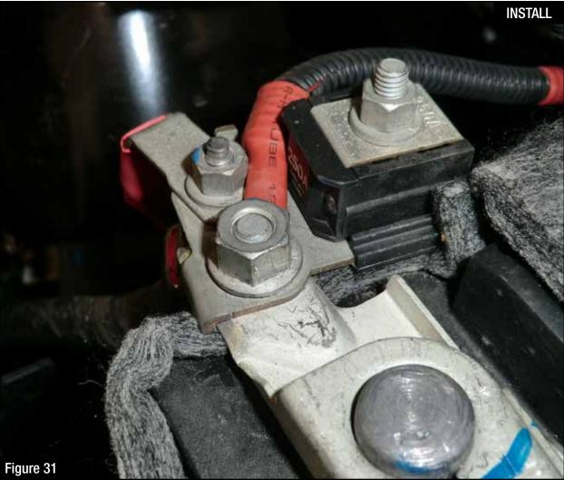
Step 46: Connect the red wire ring terminal to the positive side of the battery.
