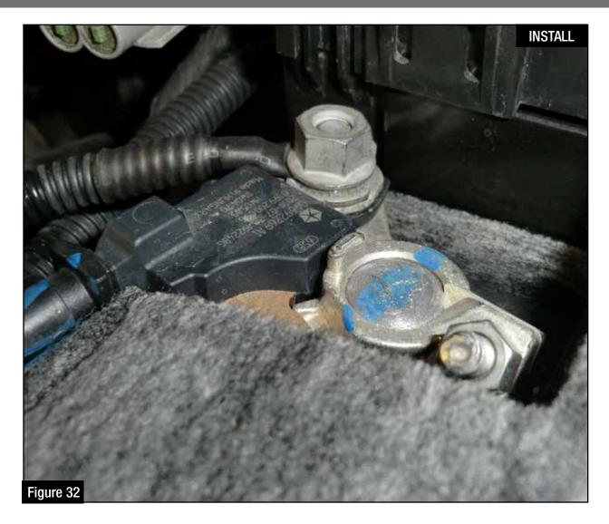
Step 47: Connect the black wire ring terminal to the negative side on the battery.
