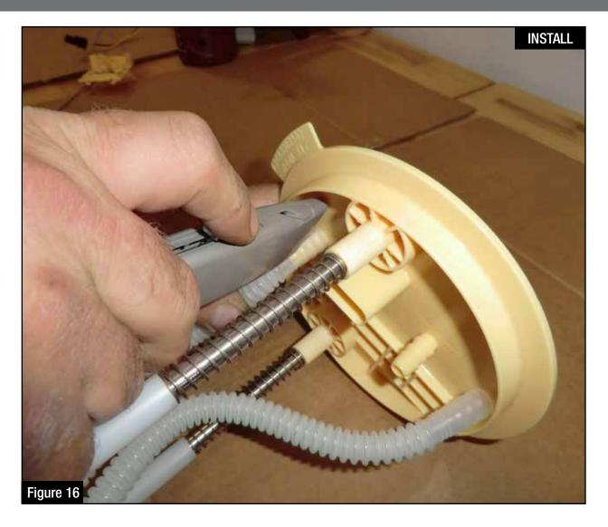
Step 20: Unplug the electrical connector at the top of the fuel pump sender assembly.
