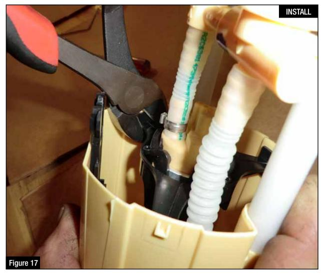
Step 23: Carefully cut the three supports for the fuel pump.
