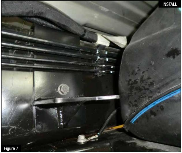
Step 8: Re-install the hard lines onto the frame rail.
