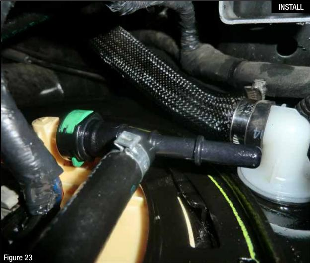
Step 33: Install the supplied fuel return line (female connection) onto the fuel pump sender assembly (male connection).
