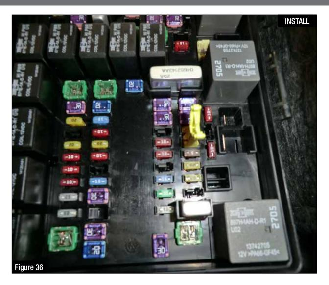
Step 52: Find a 12 volt ignition source inside the fuse box that only comes on with the key in the "run" position. The suggested fuse location is F51 "IGN MOD". Once a 12 volt source is located, pull fuse from the fuse box.
