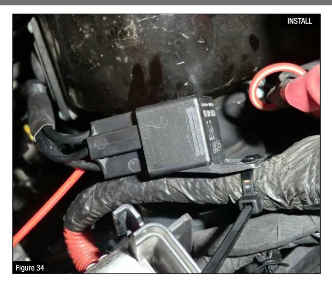
Step 50: Secure the supplied relay.
