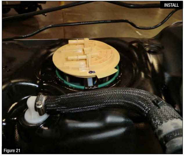
Step 30: Install the fuel pump sender assembly into the fuel tank.
