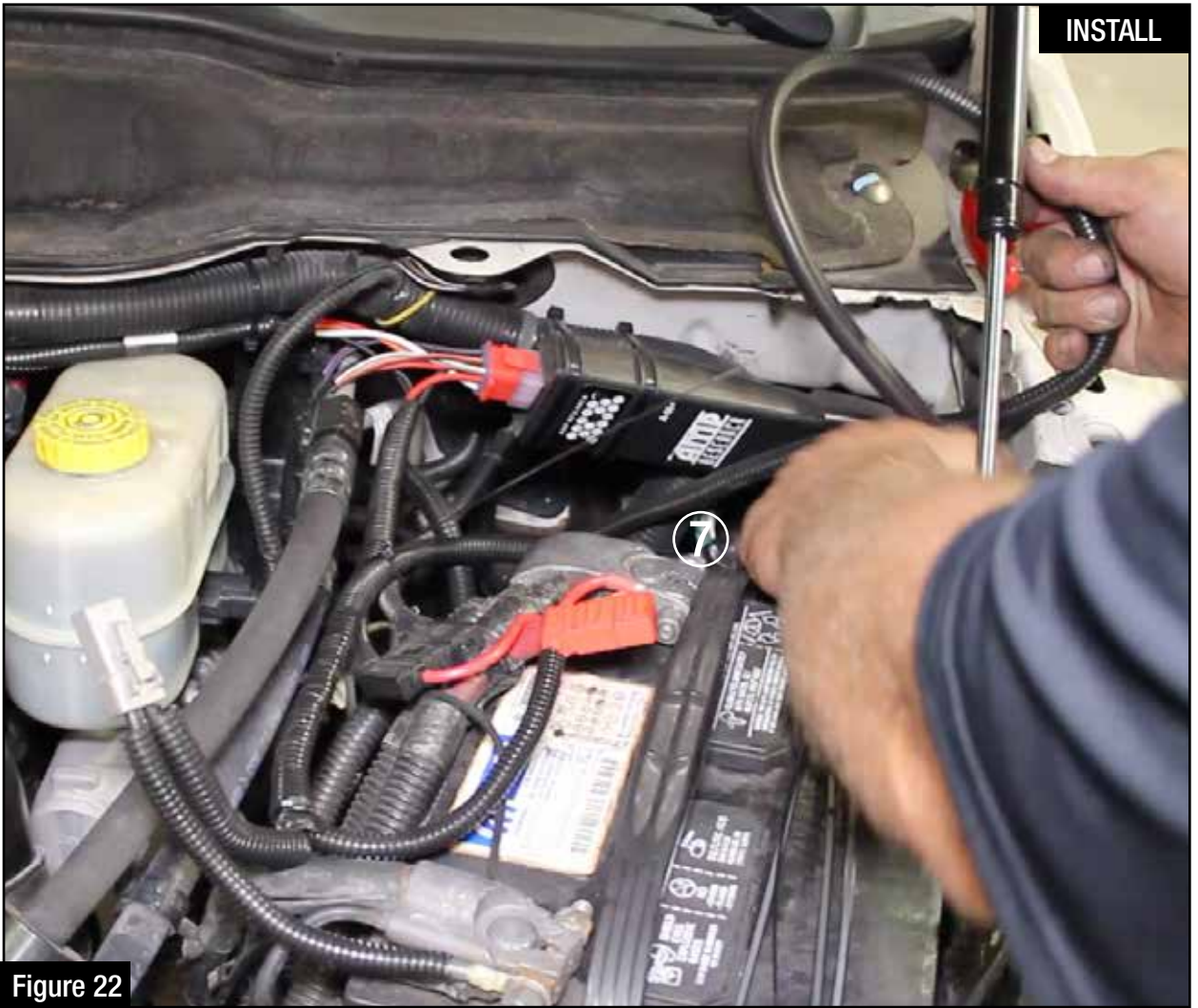
Step 27: Organize any of the loose wire harness and secure with the remaining zip ties.
