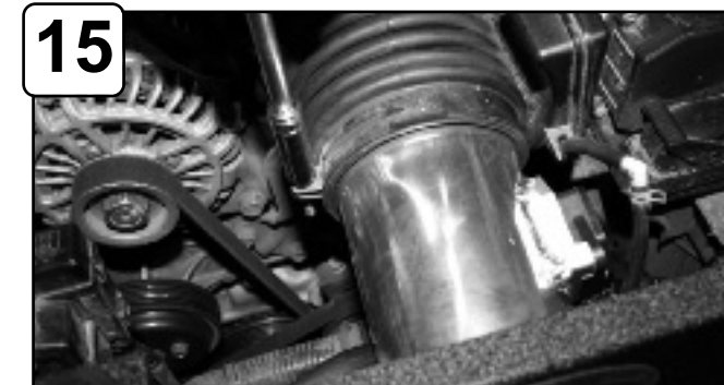
15 Tighten clamp using 10mm socket or wrench. Re-connect MAF sensor harness.
