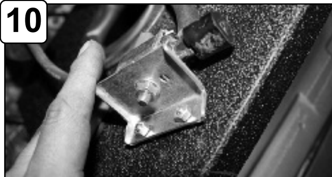
10 Attach VSV sensor to back of housing and secure using provided M4 screws and nuts.
