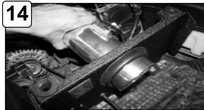
14 Install tube through back of housing and position.
