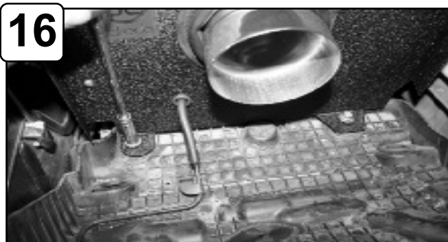
16 Tighten screws using 10mm socket or wrench.
