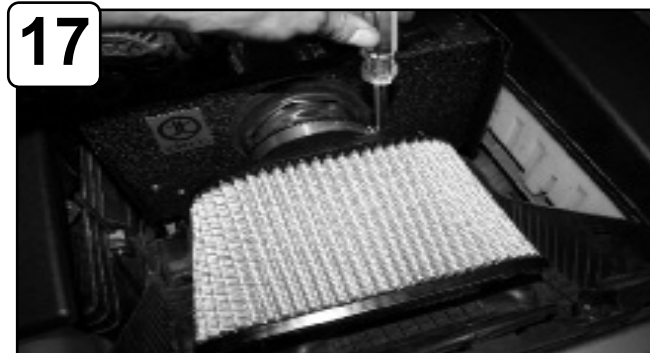
17 Install filter and tighten using 5/16" nut driver. Re-install engine cover. Re-connect battery terminals.
