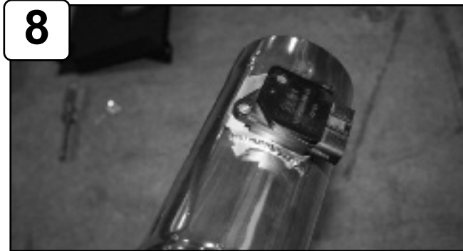
With provided M4 screws, install MAF sensor to new intake tube.
