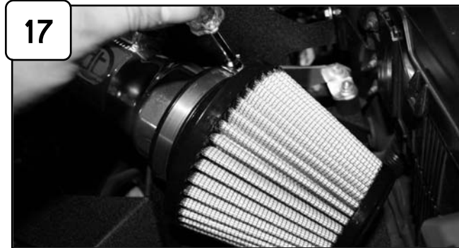
17 Install air filter and tighten using 5/16" nut driver.
