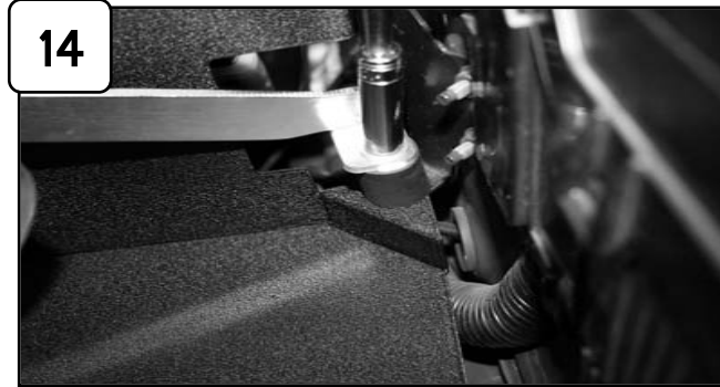
14 Tighten tab using provided Flat washer, wavy washer and nut.
