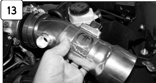
13 Install intake assembly and position tab to isolation mount. Do not tighten.
