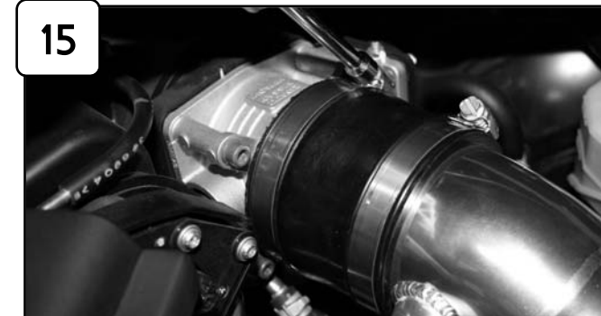
15 Tighten all clamps using 5/16" nut driver.
