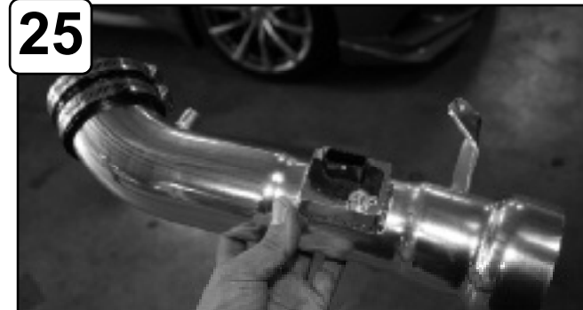
Attach coupling with clamps to tube.
