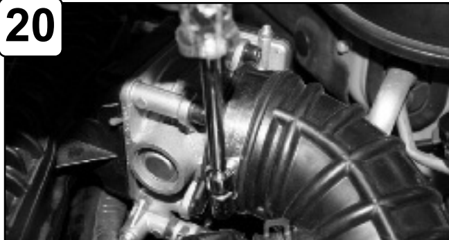
Disconnect MAF sensor harness. Loosen clamps using 5/16" nut driver.
