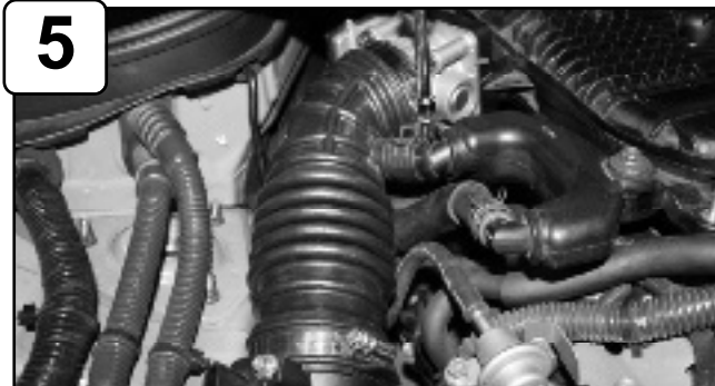
Loosen clamps on intake using 5/16" nut driver.
