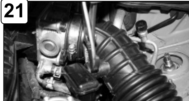
With pliers pull back stock intake tube from vent box.
