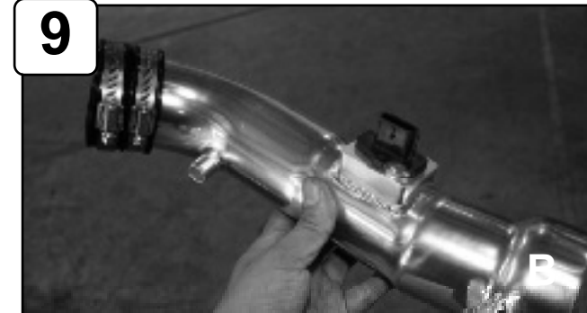
Install MAF sensor to new tube using provided M4 screws. Attach coupling with clamps to tube.
