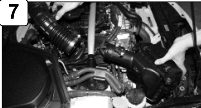
Remove complete intake out of vehicle.
