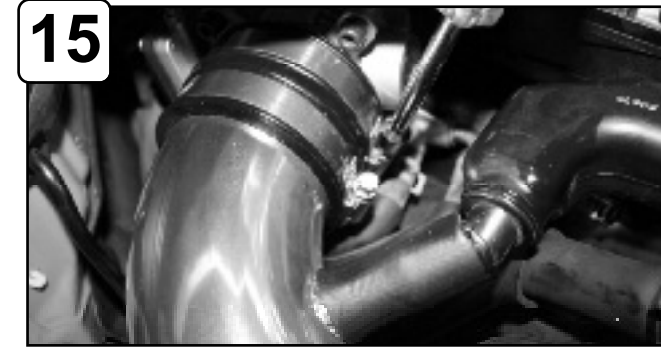
15 Tighten all clamps using 5/16" nut driver. Attach provided 5/8" hose to intake tube and plenum.
