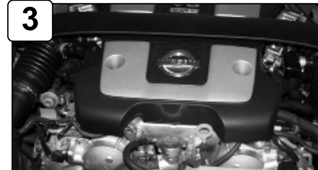
With 10mm socket or wrench, loosen the 2 bolts holding in lower engine cover and remove.
