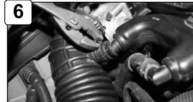
With pliers pull back crank case line from intake.
