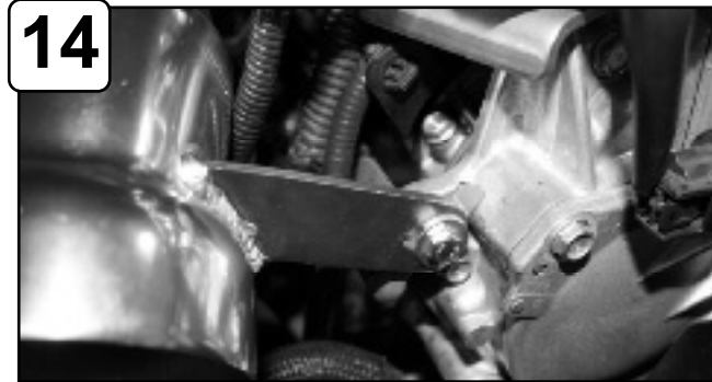
14 Secure tab to engine and tighten using provided M6 screw and flat washer.
