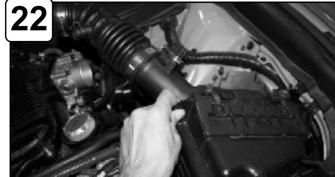
Remove complete intake out of vehicle.
