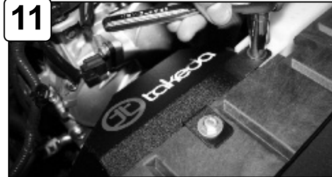
11 Install housing and secure to radiator support and tighten using bolt from previous step. Secure other tab using provided M6 screw, flat washers and nut.
