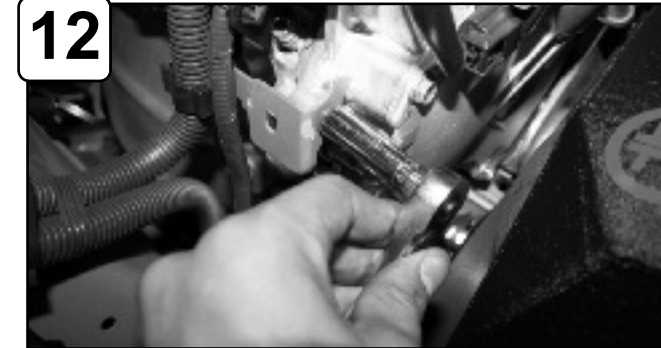
12 Loosen bolt on engine securing harness bracket.
