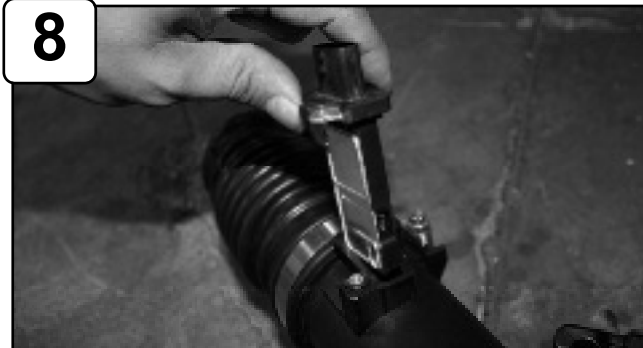
Remove MAF sensor from stock intake.
