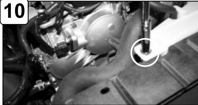
10 With 10mm socket or wrench loosen the 1 bolt on the radiator reservoir.
