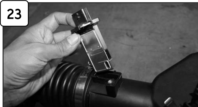
Remove MAF sensor from stock intake.
