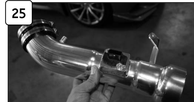
Attach coupling with clamps to tube.
