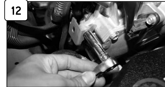
12 Loosen bolt on engine securing harness bracket.
