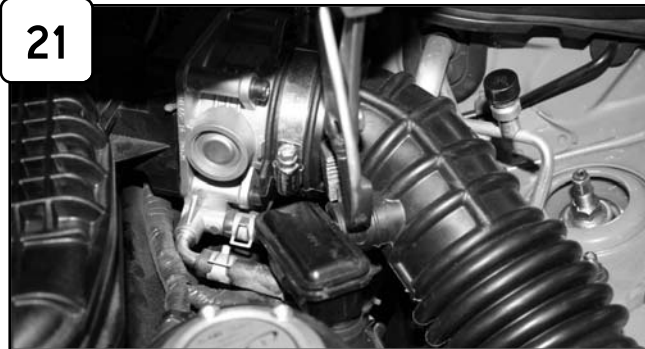
With pliers pull back stock intake tube from vent box.
