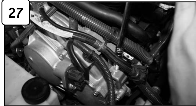
Loosen bolt on engine securing harness bracket.
