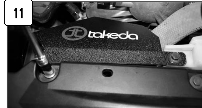
11 Install heat shield and secure to radiator support and tighten using bolts from previous step.
