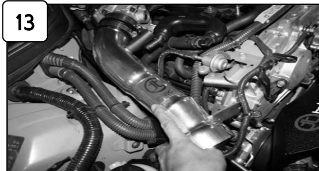
13 First re-connect MAF sensor harness. Install into vehicle and position tube. Do not tighten clamps.
