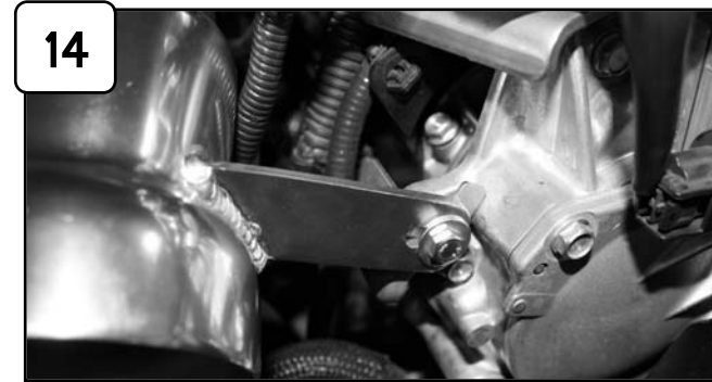
14 Secure tab to engine and tighten using provided screw and flat washer.
