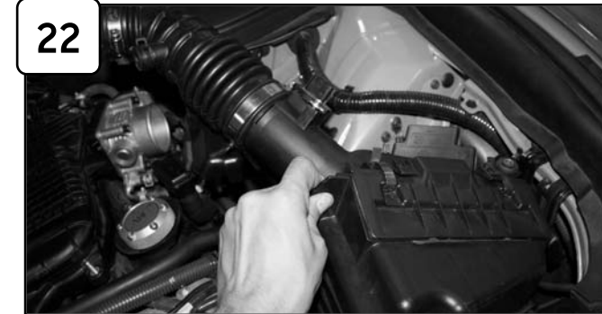
Remove complete intake out of vehicle.
