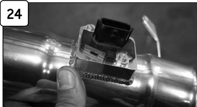
Install MAF sensor to new tube using provided M4 screws.
