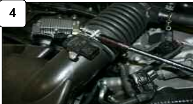
With 10mm socket and ratchet, loosen the two clamps using a 10mm socket or wrench from the OEM intake tube and airbox. Disconnect MAF sensor harness.
