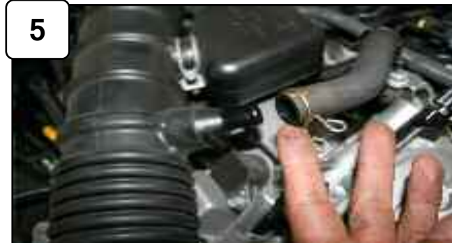
Remove crank case line from stock intake tube.
