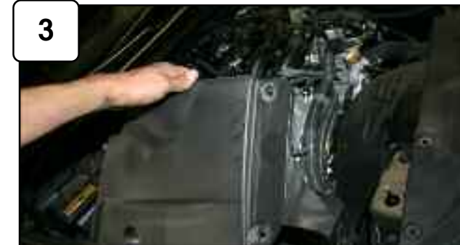
Remove engine cover and front/passenger plastic covers.
