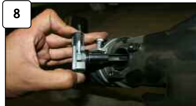
Remove MAF sensor using phillips screwdriver.
