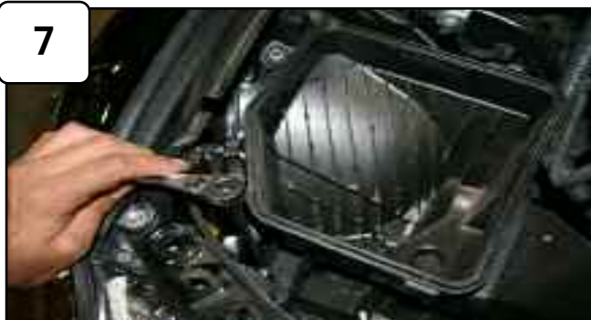
With 10mm socket or wrench loosen the 2 bolts holding in bottom half of air box and remove.
