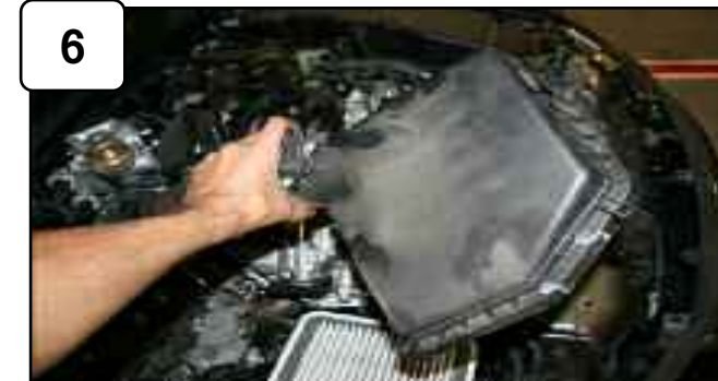
Carefully remove stock air box assembly out of vehicle.
